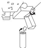
3. Remove sanitary cap from new filter.
