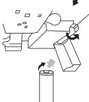
3. Remove sanitary cap from new filter.
