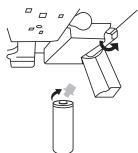
3. Remove sanitary cap from new filter.
